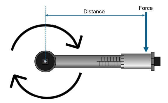
Torque (NM or Ft Lbs) = force x distance Power (kW or hp) = torque x speed Energy Consumption (kWh or hp\*h) = power x time
