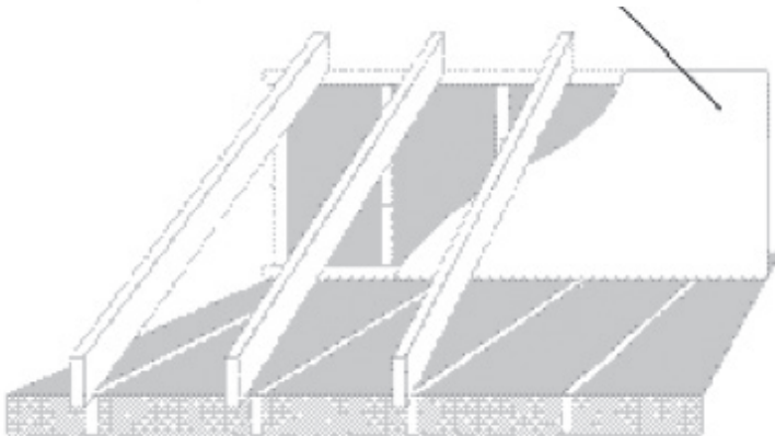
Cover knee wall with vapor-permeable air barrier
